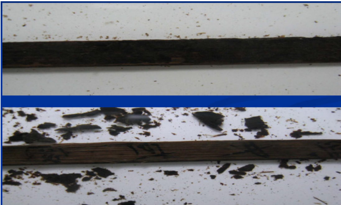
Strips before and after surface material removal.
