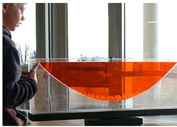
Parabolic shape formed by a liquid surface under rotation. ( Wikipedia , "Parabola")
